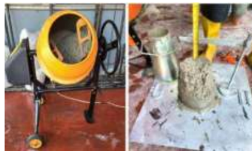
Figure-6. Measurement of workability with a slump test.
