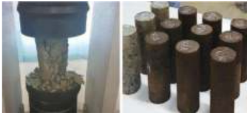
Figure-11. The compressive test process for DCT, DCL, WCT and WCL types of concrete samples.
