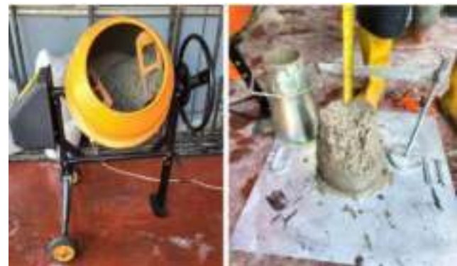
Figure-6. Measurement of workability with a slump test.
