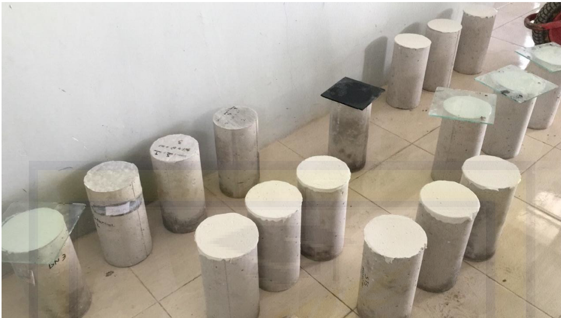
CAPPING BETON VARIASI
