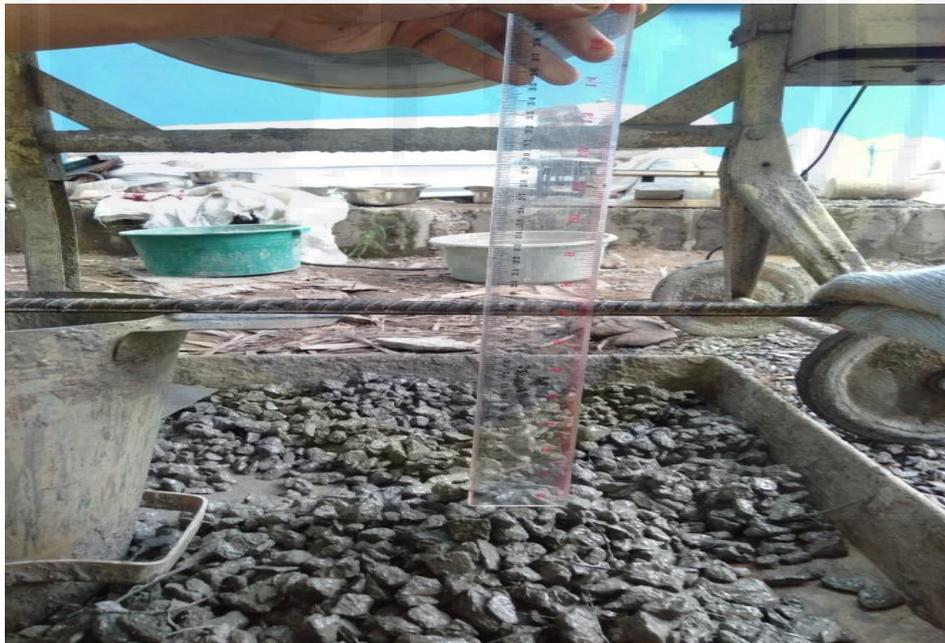
PROSES PENGUJIAN SLUMP TEST
