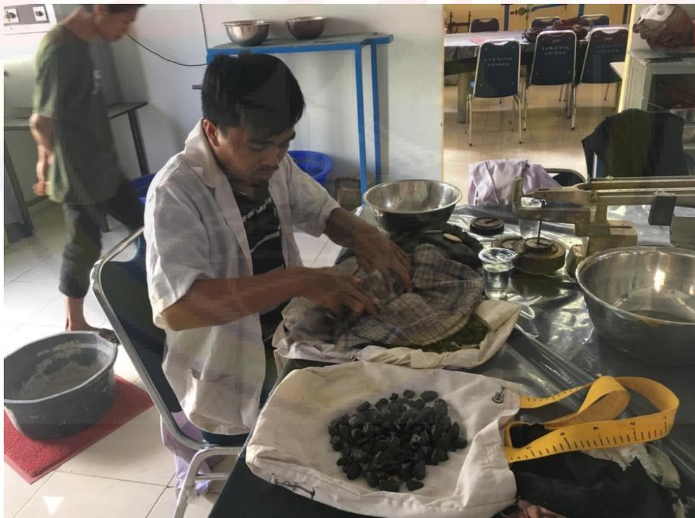
**PENGUJIAN SSD AGREGAT KASAR**
