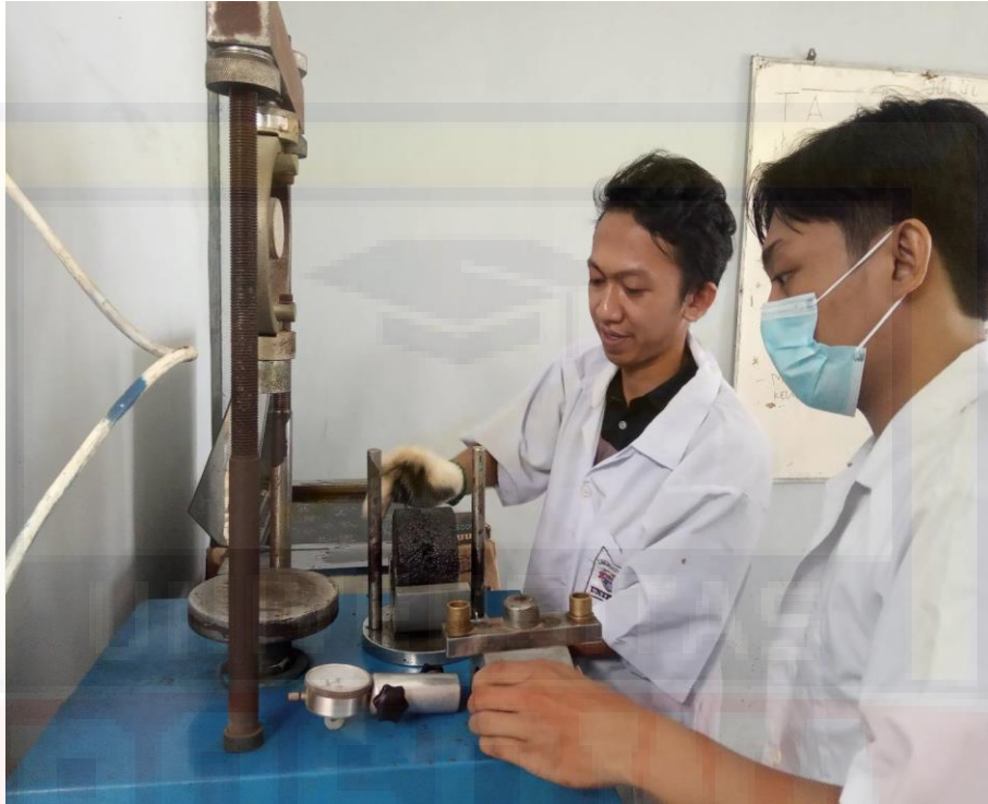
Proses Uji Marshall
