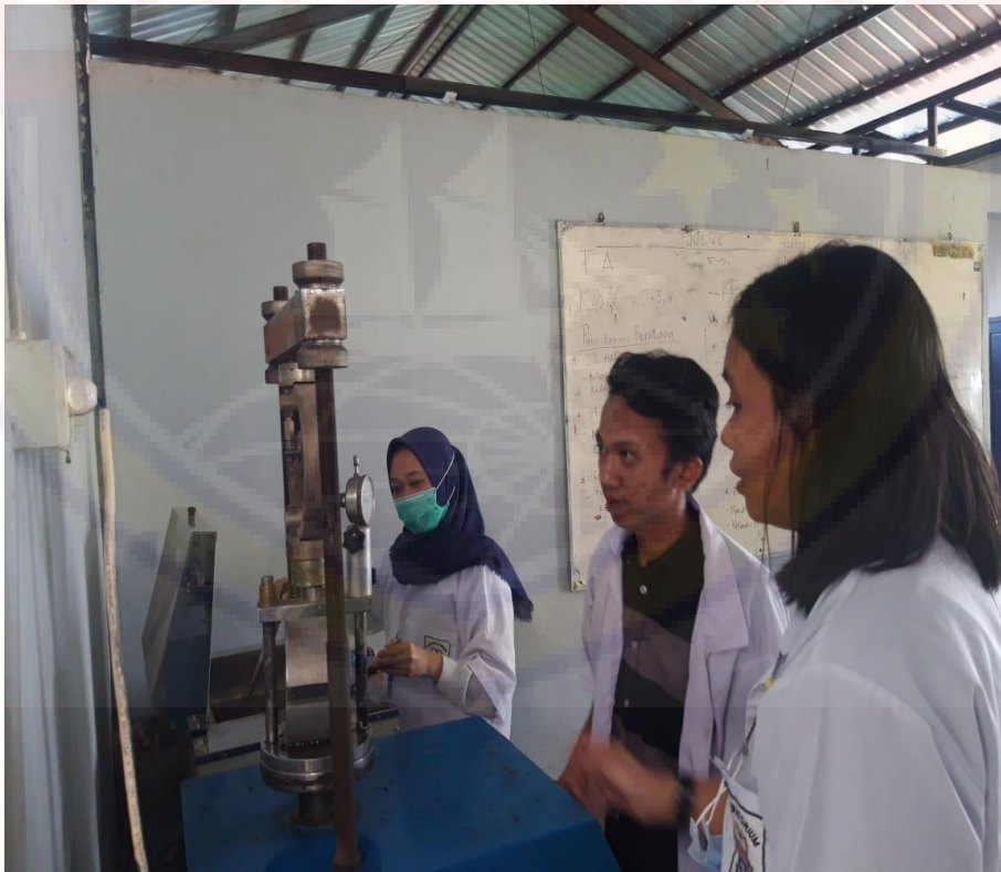
Proses Uji Marshall
