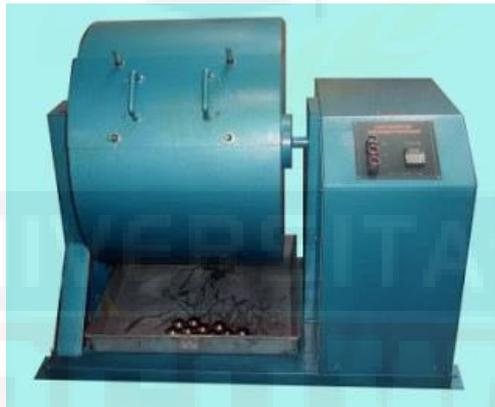
**Gambar 3.4. Los Angeles Abrasion Test**
