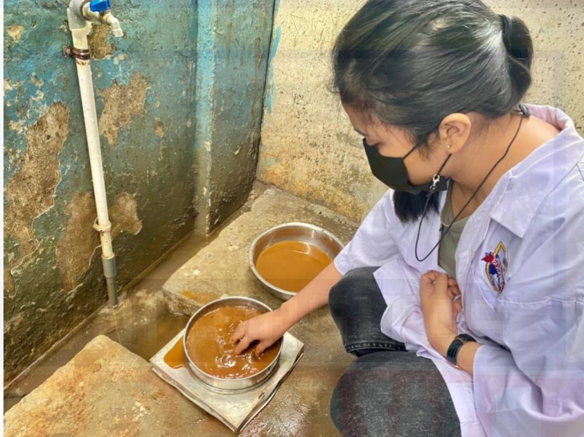
Proses pencucian sampel tanah
