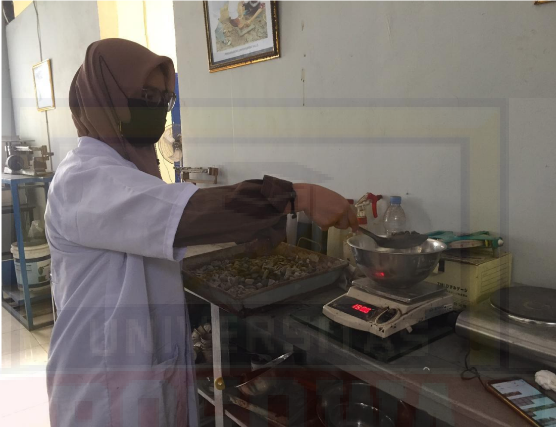
Proses Penimbangan Agregat
