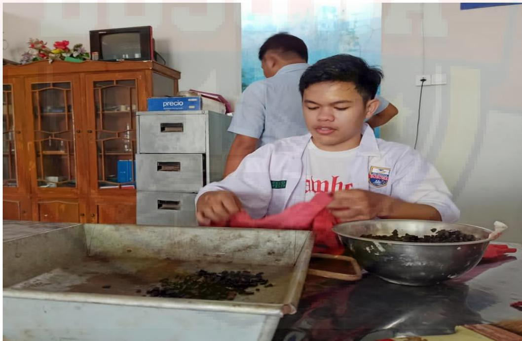
PENGUJIAN SSD AGREGAT KASAR
