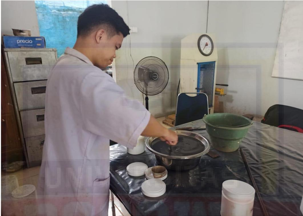
PROSES PENCAAMPURAN  $\text{NaOH}$  DENGAN  $\text{Na}_2\text{SiO}_3$  (AKTIVATOR)
