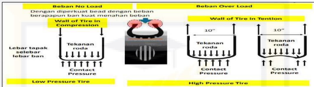
Gambar 2.5, Efek ban terhadap beban overload (Sumber : Roadmap and Refleksi Odol)
