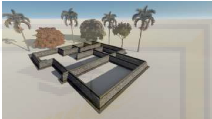
Gambar III.26 Pondasi Batu Kali
