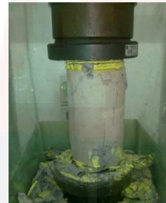
(a) f'_c=31.3 Mpa (b) f'_c=52 Mpa (c) f'_c=77.7 MPa Gambar
