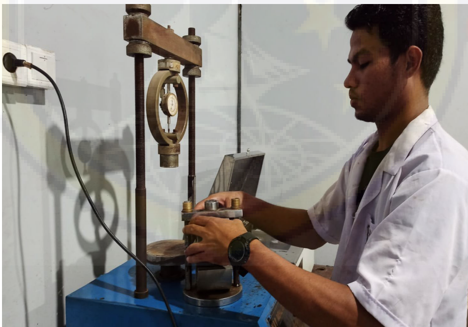
Proses Uji Marshall
