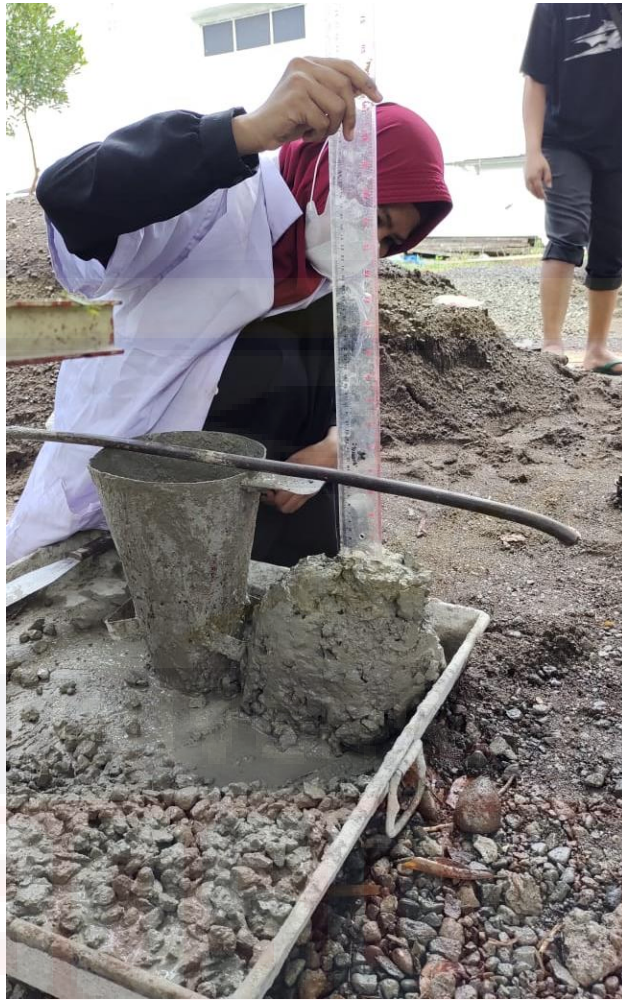
HASIL SLUMP TEST
