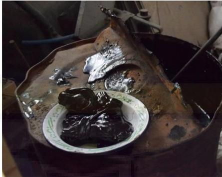
Gambar 3.5 Aspal Minyak Penetrasi 60/70
