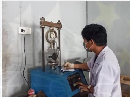
Gambar 3.7 *Marshall Test Machine*
