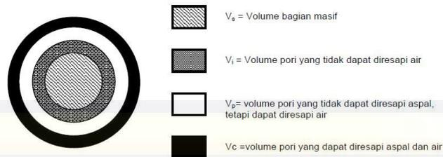
Gambar 2.5 Skema Volume Butir Agregat
