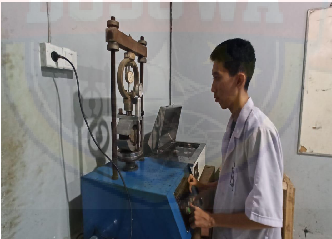
Proses Uji Marshall
