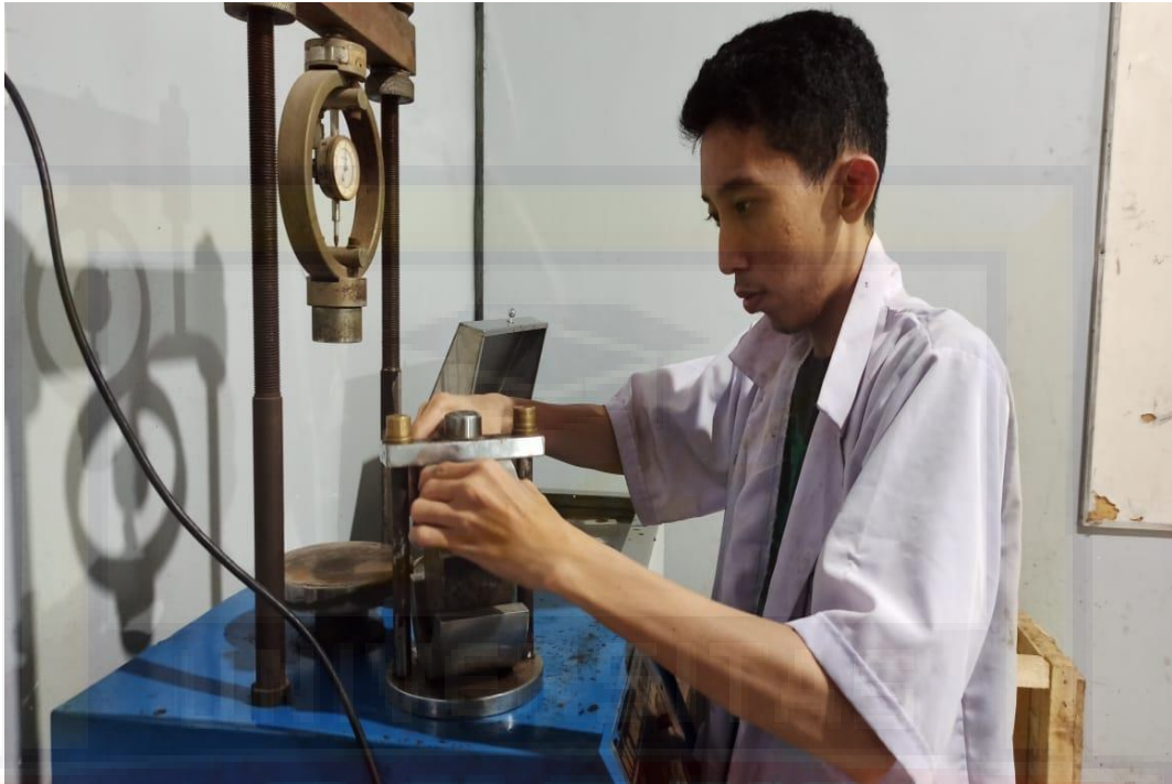
Proses Uji Marshall
