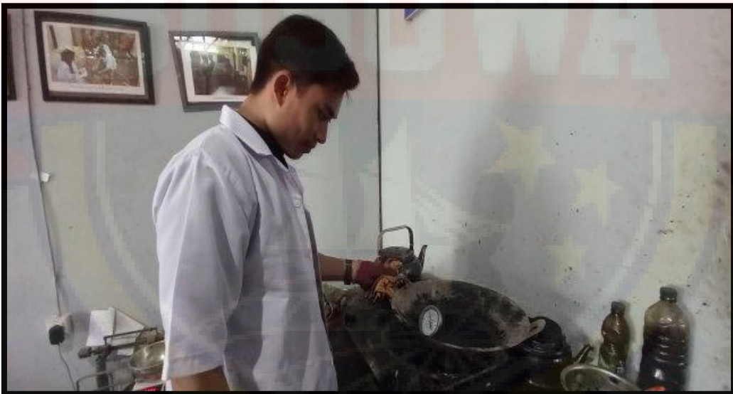
Pengecekan Suhu Campuran Aspal
