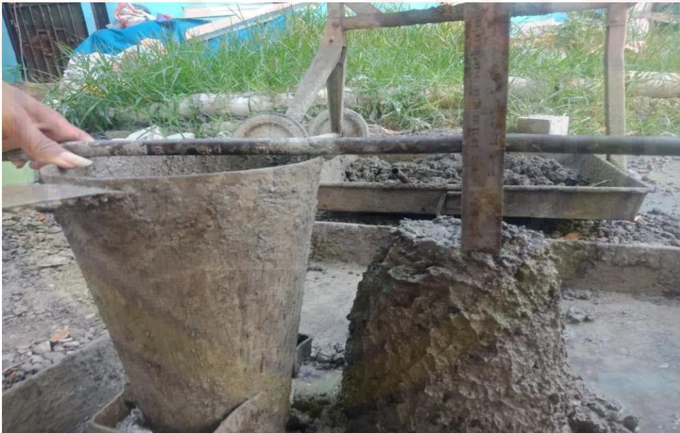
PENGUJIAN SLUMP TEST
