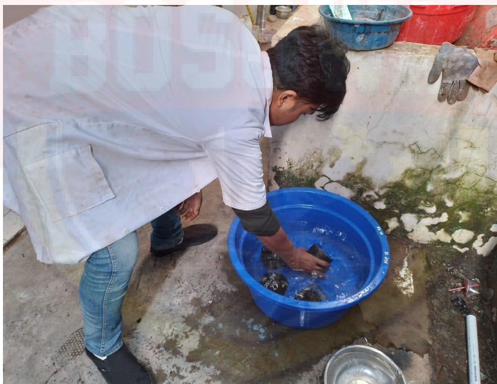
Gambar 1.14. Proses Perendaman Briket
