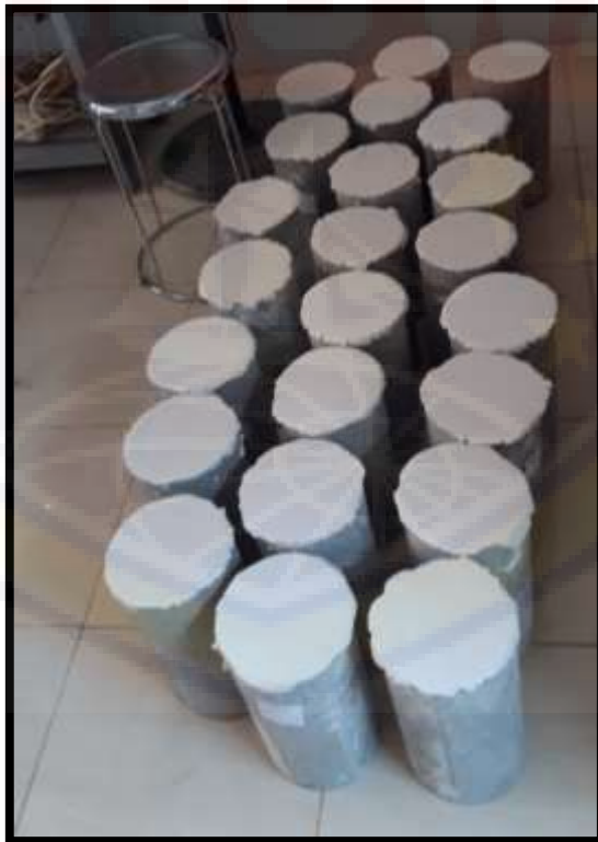
Gambar 20. Proses Kepping Sampel Beton
