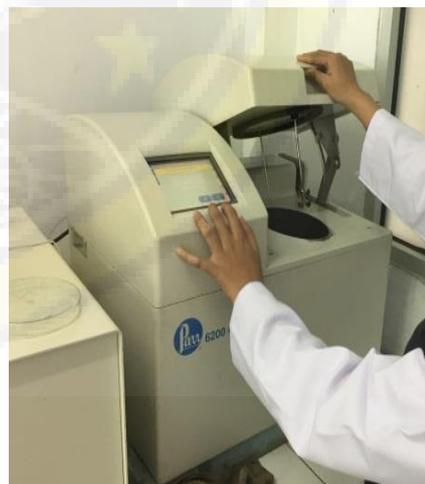
**Gambar C.4:** Bomb Calorimeter (Analisa Nilai Kalori (kcal/g))
