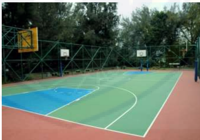
Gambar 2.10: Lantai Arcylic Surfacing Sumber: www.njpssportscourts.com , 2017
