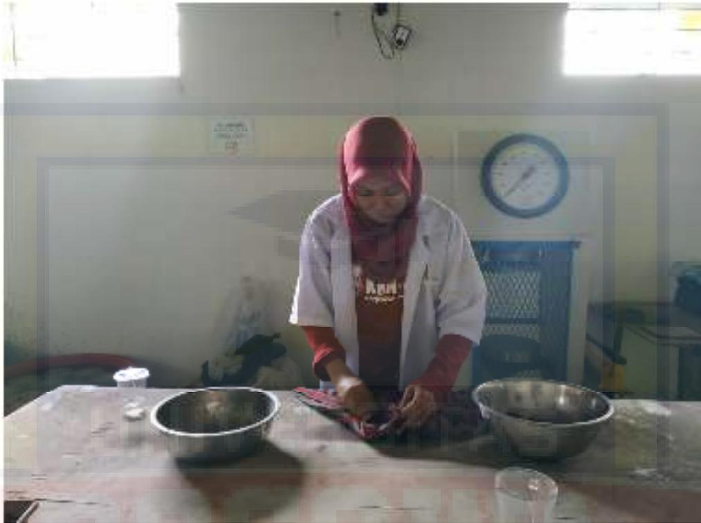
**PENGUJIAN SSD AGREGAT KASAR**
