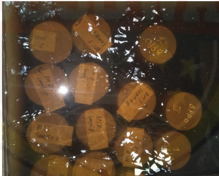
PROSES PERENDAMAN BETON
