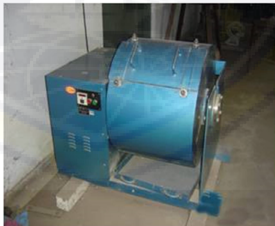
Gambar 3. 5 Los Angeles Abrasion Test
