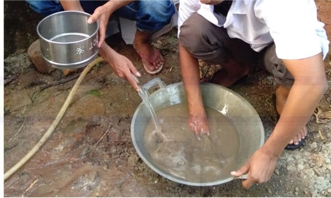
Gambar 3. 6 Pengujian kadar lumpur agregat kasar
