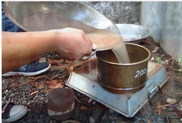
Gambar 3. 7 Pengujian kadar lumpur agregat halus
