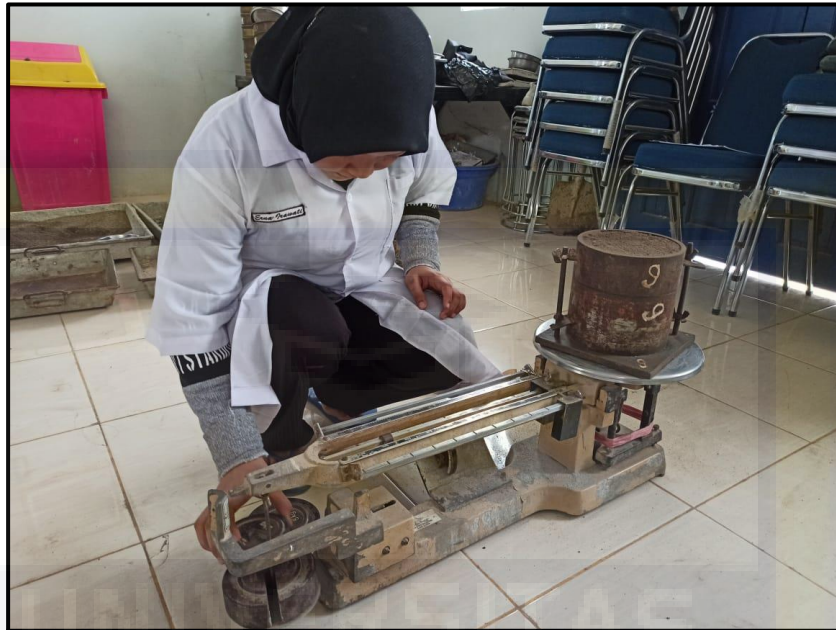
Gambar 4.15. Menimbang benda uji (agregat halus)
