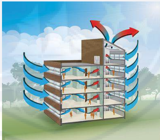
Gambar 4.24 sistem penghawaan bangunan Sumber: https://www.arsitur.com/2017
