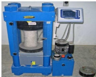
Fig.2. Concrete Compressive Test Machine
