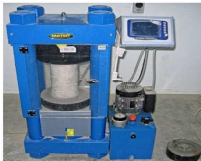
Fig.2. Concrete Compressive Test Machine
