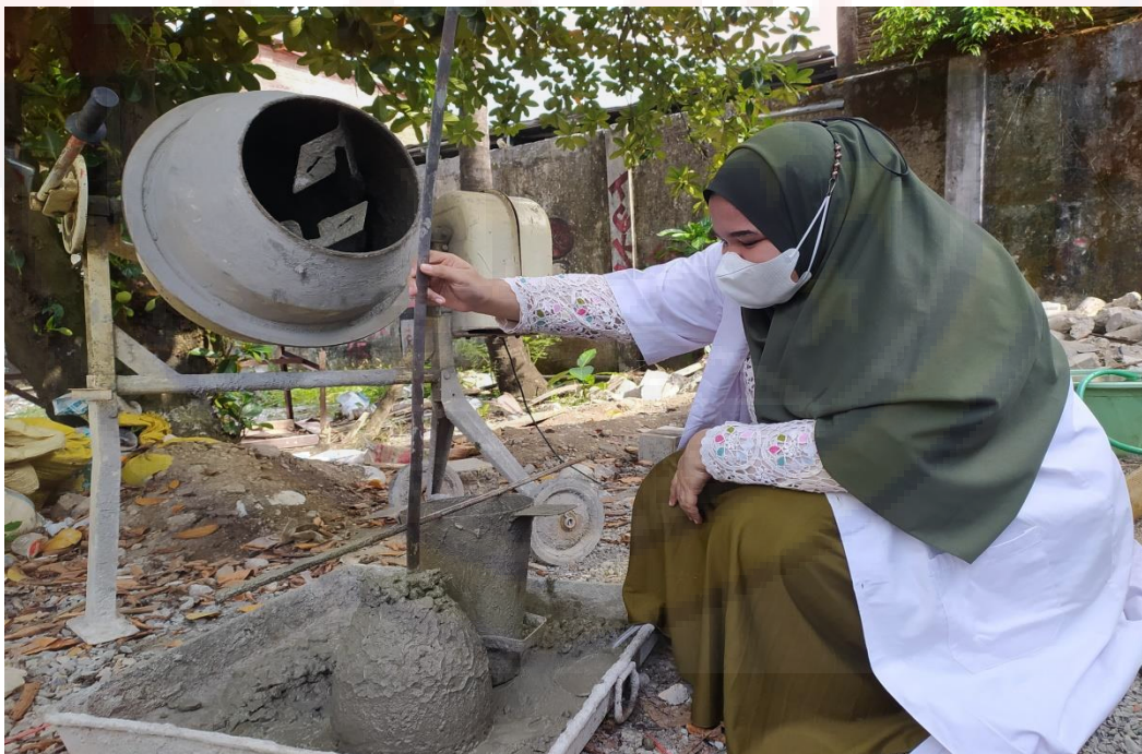
Gambar 8. Proses Test Slump Beton
