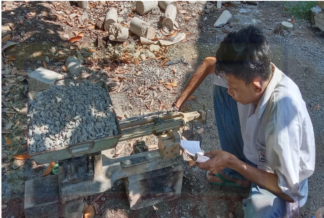
Proses Penimbangan Agregat Kasar
