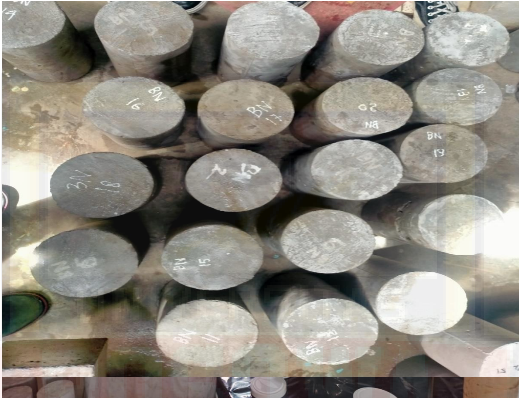
BENDA UJI BETON NORMAL
