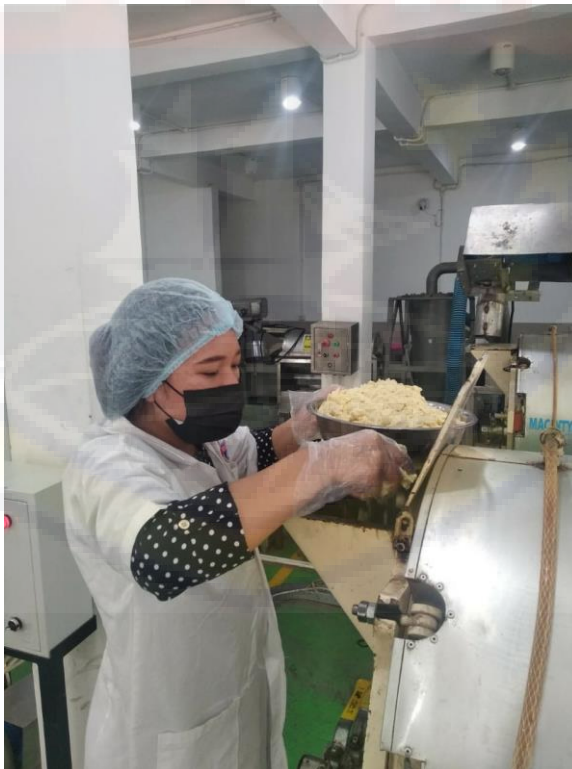
Gambar 4. Proses Conching Lemak Cokelat
