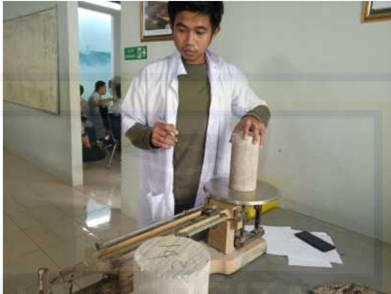
PENIMBANGAN BERAT BETON KERING (SILINDER)
