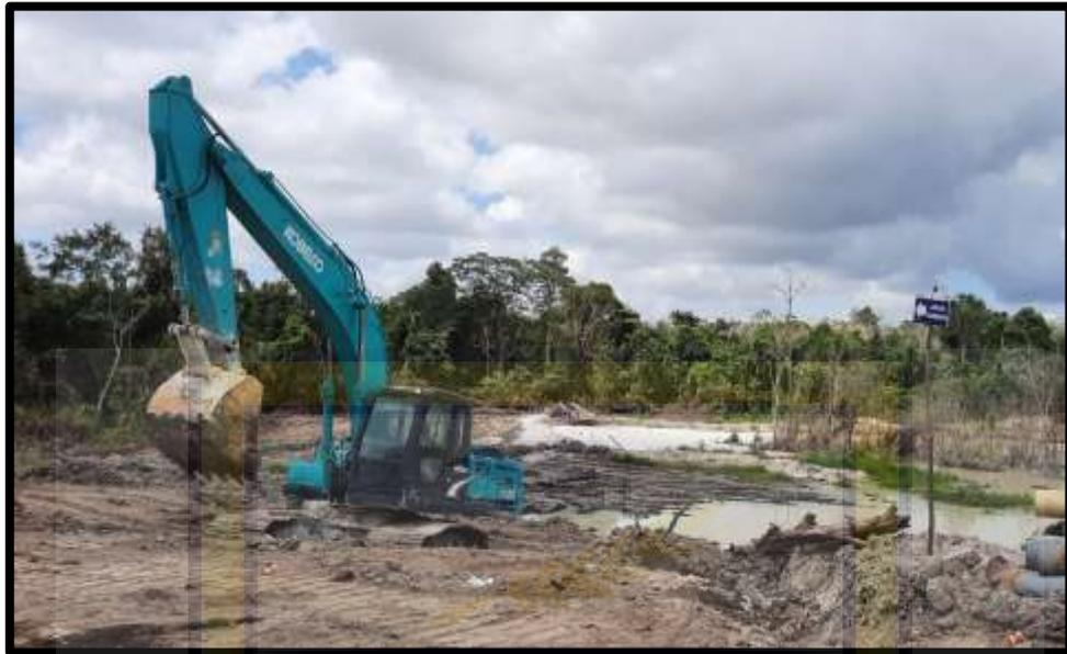
Gambar J. 3 Alat Berat Excavator Kobelco SK200
