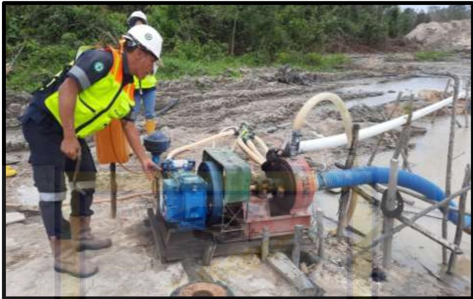
Gambar J. 5 Mesin Pompa Semprot Dongfeng
