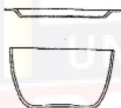
FIG. 2 Capsule for Use in Determining Moisture
