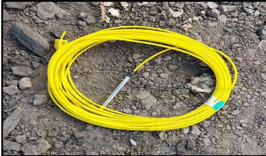
**Gambar 2.14** *Detonator In Hole Delay* ( PT. Petrosea Kbl site Ccm )
