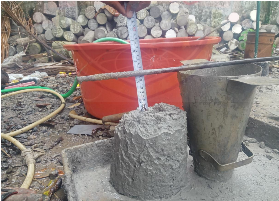
Pengambilan Nilai Slump Test beton normal
