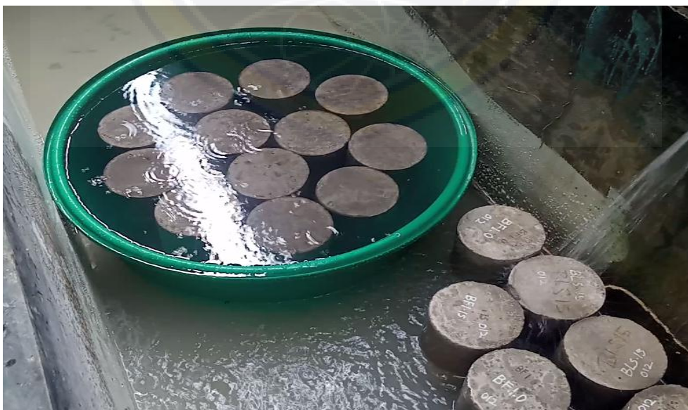
Perendaman Beton Normal
