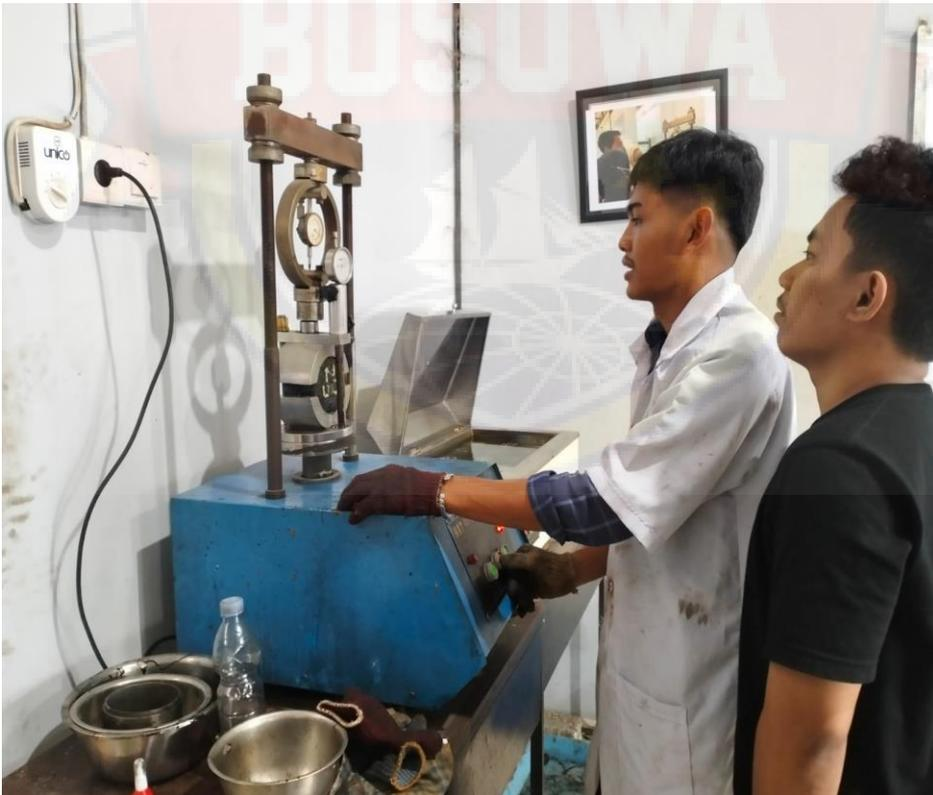
**Proses Uji Marshall Test**
