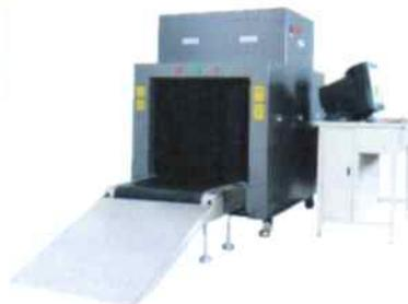
Gambar 2. 7 : Metal Detector X-ray
