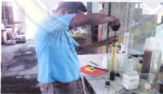
Selasa 12-04-2011 Jam 12.51 Uji Sand Equivalent
